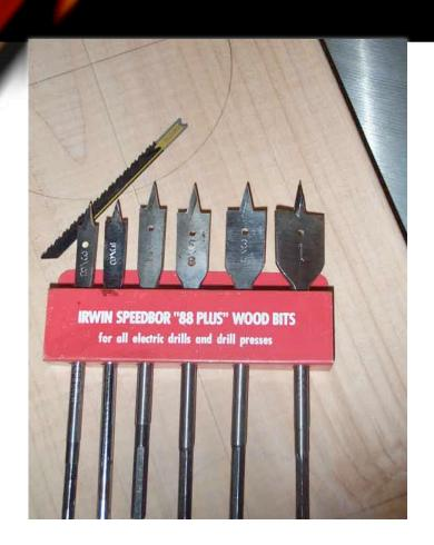
© Use a "spade" bit to get a pilot hole that will fit the required sabre saw blade. 3/8" works fine here, and allows about the narrowest sabre blade that will cut "2-by" stock without breaking.
