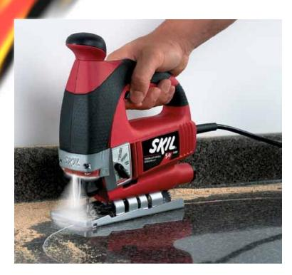
The sabre saw is the best hand tool for cutting curves and making inside cuts. Make sure you use the correct blade: narrow for curves, wide for straight cuts. Big teeth for fast/rough cuts, smaller for finer cuts.
