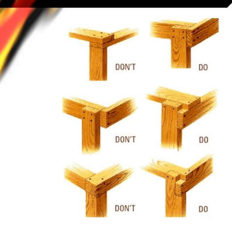
These pictures show how you can use simple, square-cut boards to make strong screw 'n glue joints, avoiding end-grain problems.
